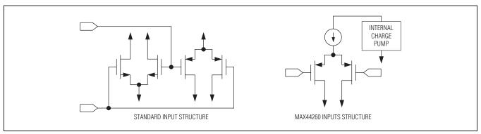
Figure 1. Comparing the Input Structure of the MAX44260 to Standard Op-Amp Inputs
