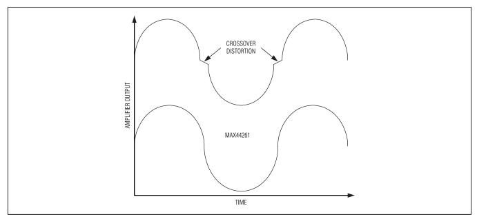
Figure 2. Crossover Distortion of Typical Amplifiers
