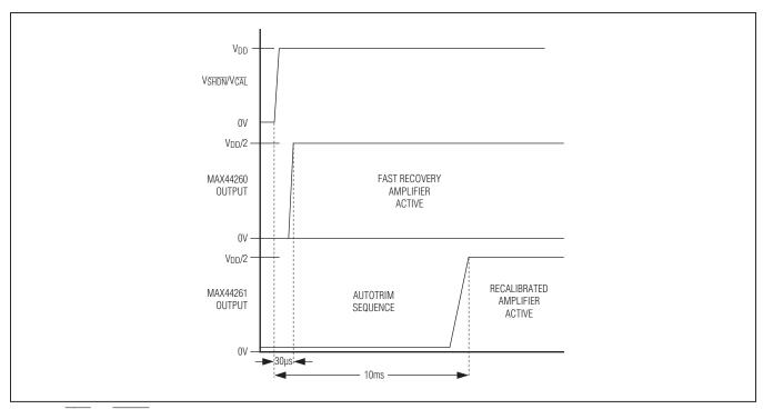
Figure 3. CAL vs. SHDN Input Operation
